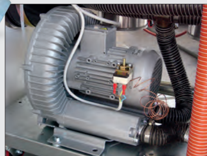
High performance side channels blowers 高性能側通道鼓風機
