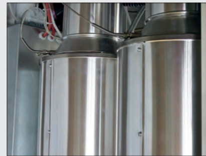
Two molecular sieves towers, high production, made of stainless steel and insulated 兩個分子篩塔，高產能，由不銹鋼製成且絕緣
