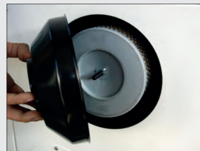
Filters with large filtering surface 大型過濾面的過濾器
