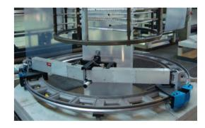
The capacitive sensor, on slewing ring, goes around the bubble and measures the film thickness along the circumference, over the frost line.
